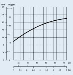
\* Clip-on models have approx. 0,5 m<sup>3</sup>/h higher flow rate Pressure/Flow
